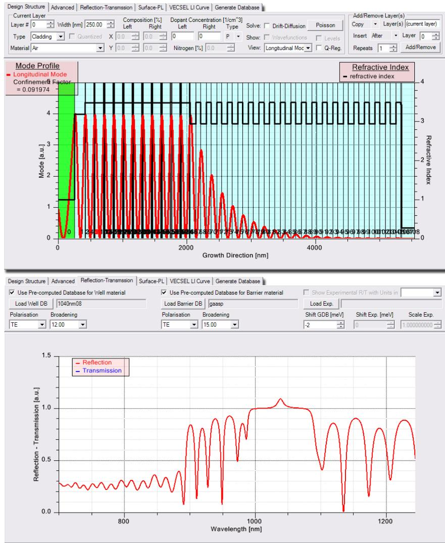
Figure 15: Top: Refractive index profile and longitudinal (propagating) mode for the full  $1040\text{ nm}$ -VECSEL structure at  $375\text{ K}$ ,  $1040\text{ nm}$  and a density of  $5 \times 10^{12}/\text{cm}^2$ . Bottom, reflection for the same conditions.
