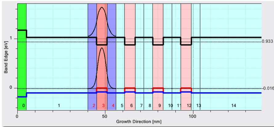
Figure 2: Undoped quantum well and cladding layers of the edge emitting device. The 'quantized region' (layers 1 2 3) is shown in darker blue and pink. The *InP*-layer '0' has been added temporarily to check for strain.
