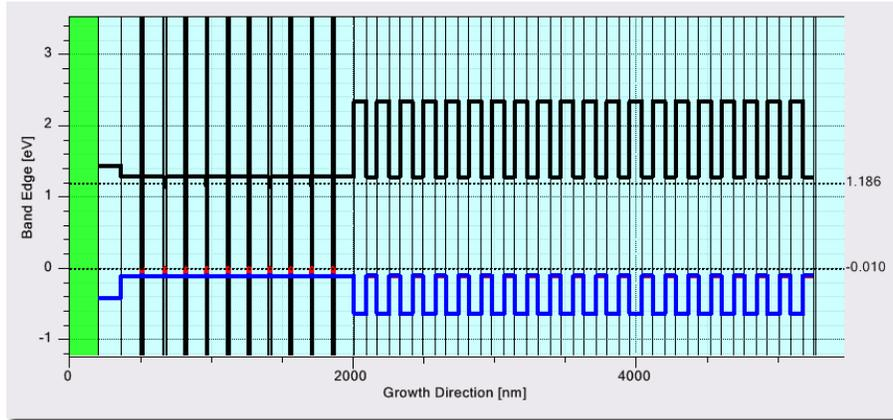
Figure 12: Confinement potential for the full 1040 *nm*-VECSEL structure.
