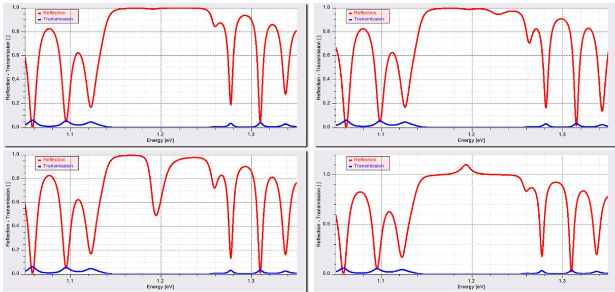
Figure 16: Reflection and transmission spectra of the 1040 nm-VECSEL. Top left: 375 K, without a database for the well. Top right: 300 K, with well-database and zero carrier density. Bottom left: 375 K, with well-database and zero density. Bottom right: 375 K, with well-database and a density of  $5 \times 10^{12}/\text{cm}^2$ .
