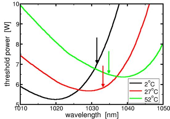
Figure 23: Threshold power for the 1040 *nm*-VECSEL as function of the lasing wavelength. Arrows indicate the actual lasing wavelengths. Data calculated using 'Tools | Current Calculator' and rescaled according to Eq.(13).
