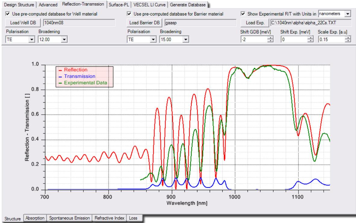
Figure 18: Comparison between experimentally measured and calculated reflectivity spectra for the 1040 nm VECSEL at 22°C and very weak excitation using **SimuLase<sup>TM</sup>**’s **’Reflection-Transmission’**-tool.
