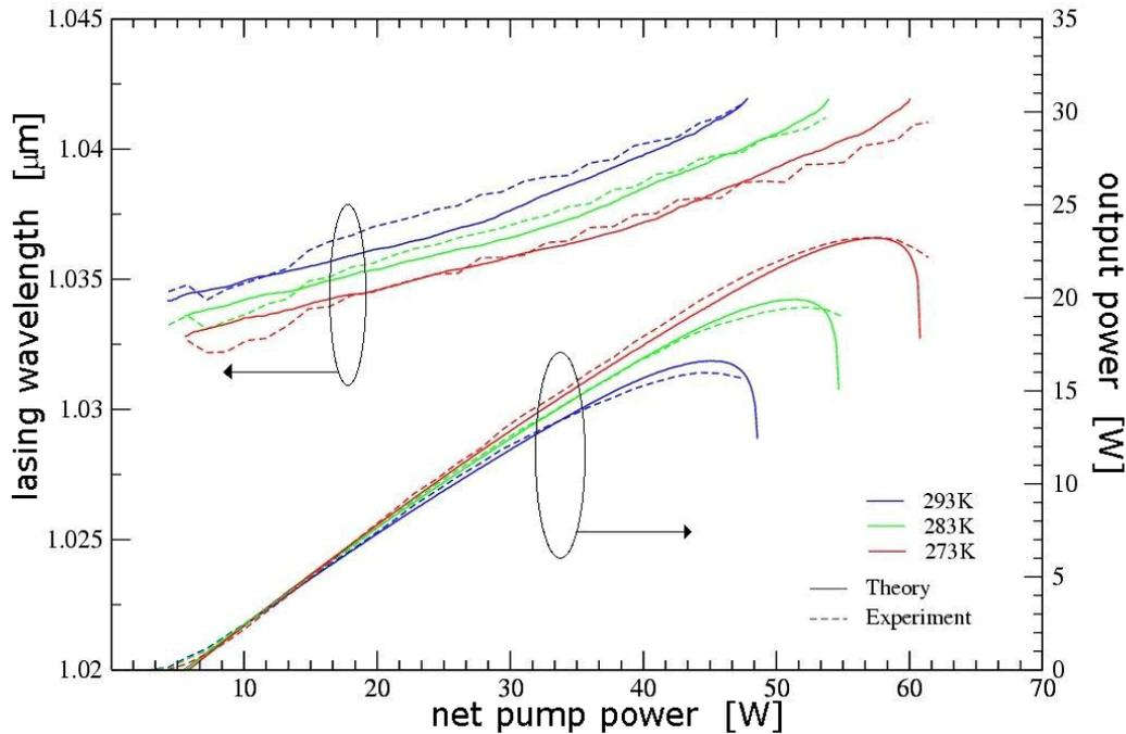
Figure 26: Comparison of theoretical and experimental output powers and wavelength shifts for the 1040 *nm*-VECSEL. Theoretical data calculated with and exported from **SimuLase**<sup>TM</sup>.
