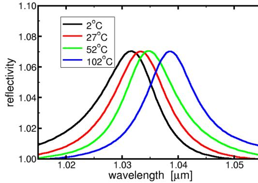
Figure 22: Calculated reflectivity at threshold carrier density for the  $1040 \text{ nm}$  VECSEL at various temperatures. (Data calculated with and exported from **SimuLase**<sup>TM</sup> .)
