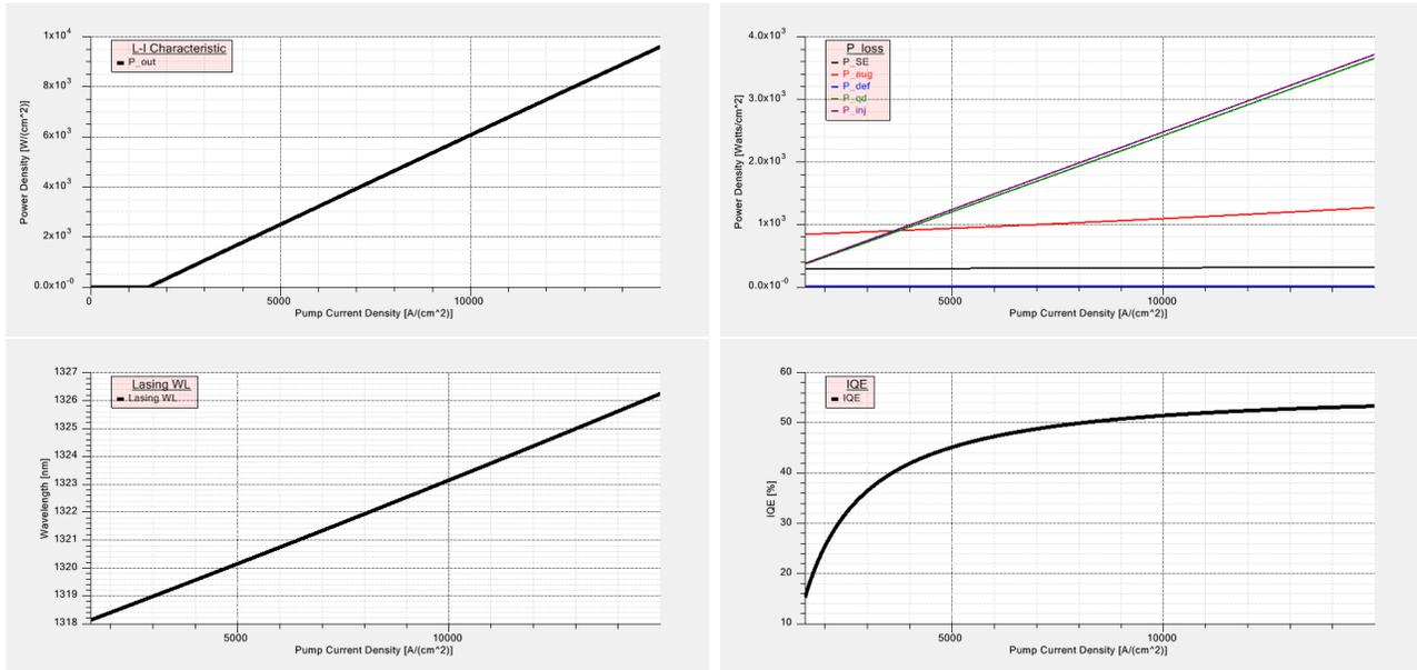
Figure 9: Operating characteristics calculated using the 'Current Calculator' tool assuming an injection efficiency of 80%, a thermal impedance of  $0.3 \text{ mm}^2 \text{ K/W}$ , a heat sink temperature of 293K and an optical loss of 1278/cm. Top left: output power. Top right: various power losses. Bottom left: lasing wavelength. Bottom right: internal quantum efficiency.
