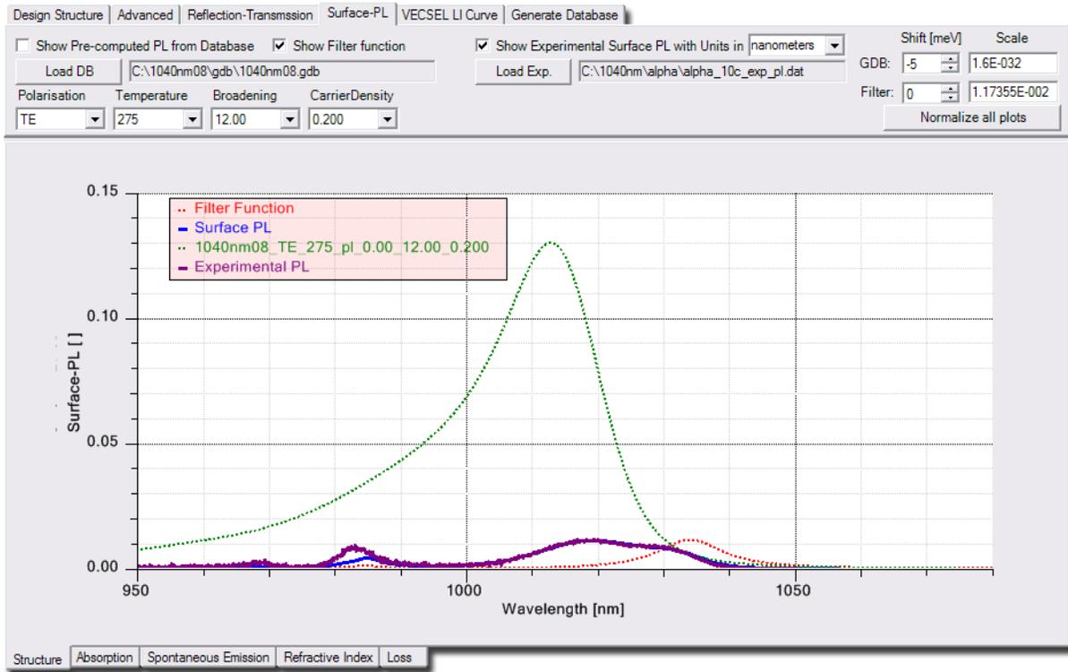
Figure 20: Comparison between experimental and calculated surface-PL spectra for the 1040 nm VECSEL at 10°C using **SimuLase**<sup>TM</sup>’s **’Surface-PL’**-tool.
